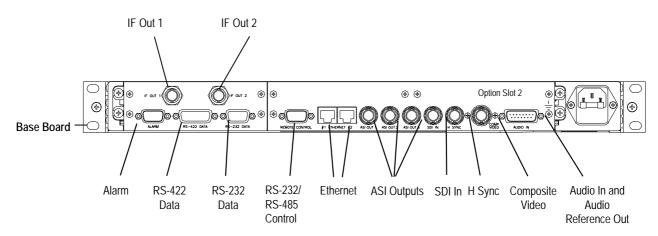
Figure 2.4: E5715 (1U) Rear Panel Component Parts and Connectors
